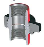
Figure 400 features a precision ball and cone sealing surface for sure metalto-metal seal. Recommended for water, oil and gas service to 4,000 PSI NSCWP.
