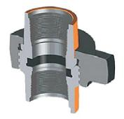
Figure 602 has a replaceable lip-type seal ring of Buna-N specifically designed to minimize fluid flow turbulence. The replaceable lip-type ring also provides a pressure seal and protection for the metal-to-metal seating surfaces. These unions are recommended for manifold and truck mounting where size and weight are critical. Recommended for air, water, oil, gas or mud service up to 6,000 PSI NSCWP.
